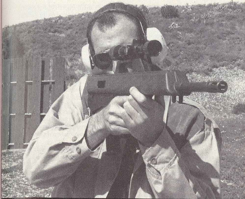
The author found the M-17S quite comfortable to fire. With the weight massed at the butt, the M-17S has less muzzle weight, reducing shooting fatigue.
